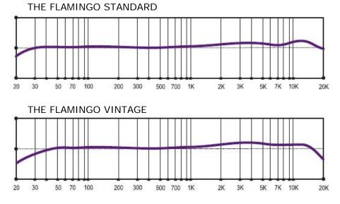
The above diagrams provide some technical information, but how the microphone reacts in concrete application depends on a number of factors - room volume, reflections, reverberation, microphone distance and the angle from the sound source and room walls, microphone external preamplifier input impedance and electronics type, microphone cable length and quality, etc. The basis of the sound comes from the know-how of the artist and engineer!
